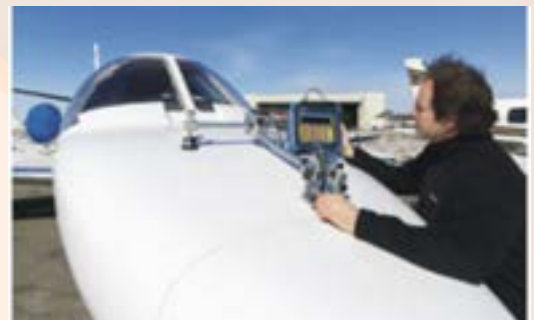
Corrosion Mapping and Composite Inspection
