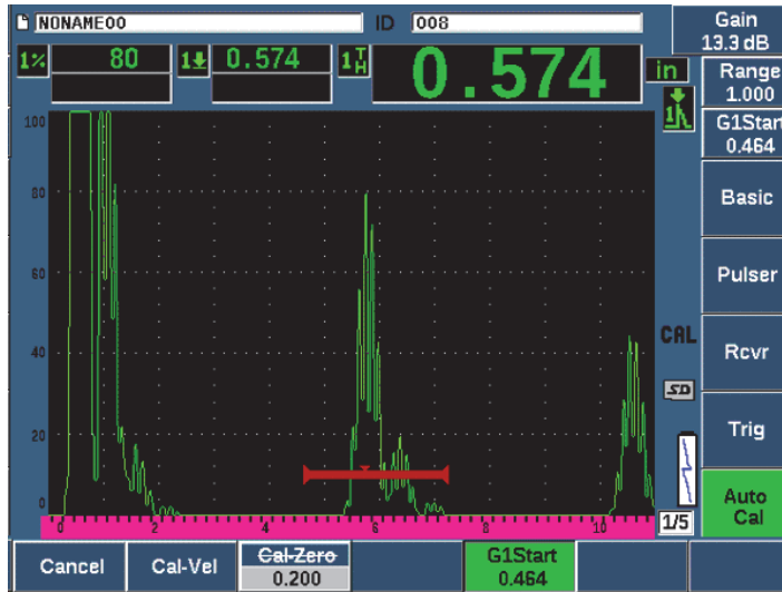
Figure 9-3 Example of a gated signal for velocity calibration
