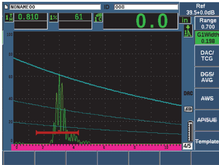
Figure 11-8 A small range DAC
