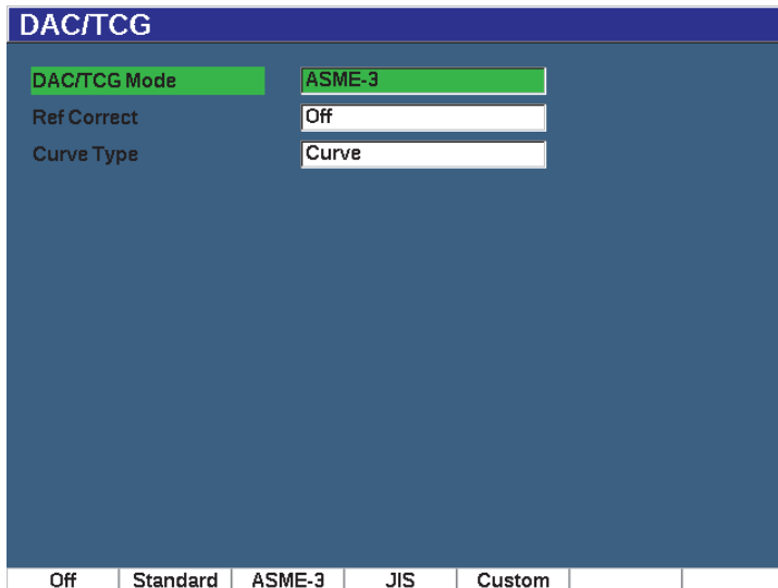
Figure 11-2 The DAC/TCG setup page
