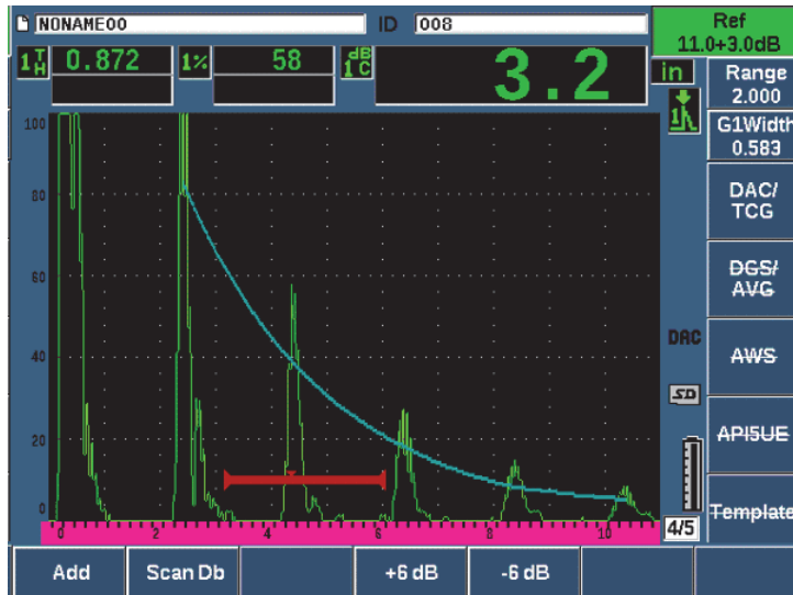
Figure 11-9 Standard DAC with 3 dB scanning gain
