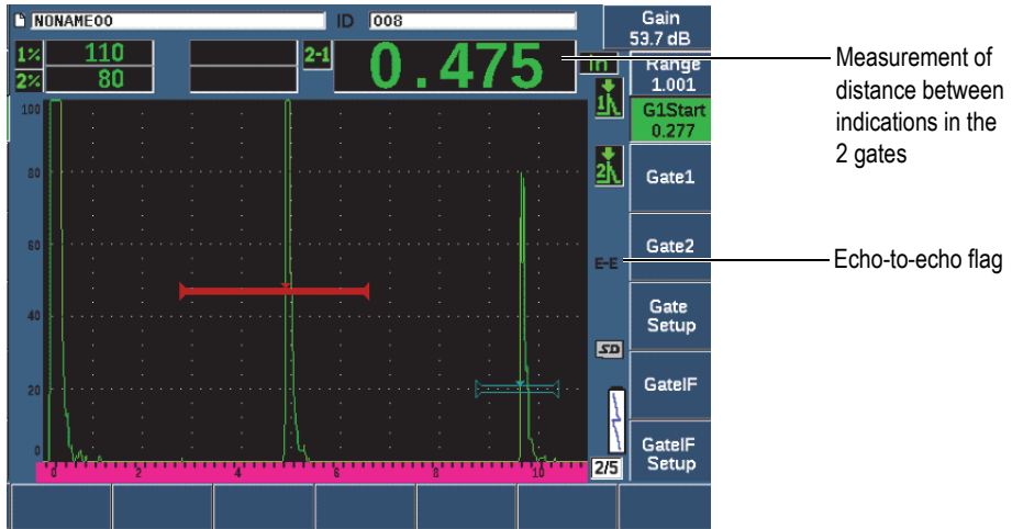
Figure 7-7 Echo-to-echo measurement example
