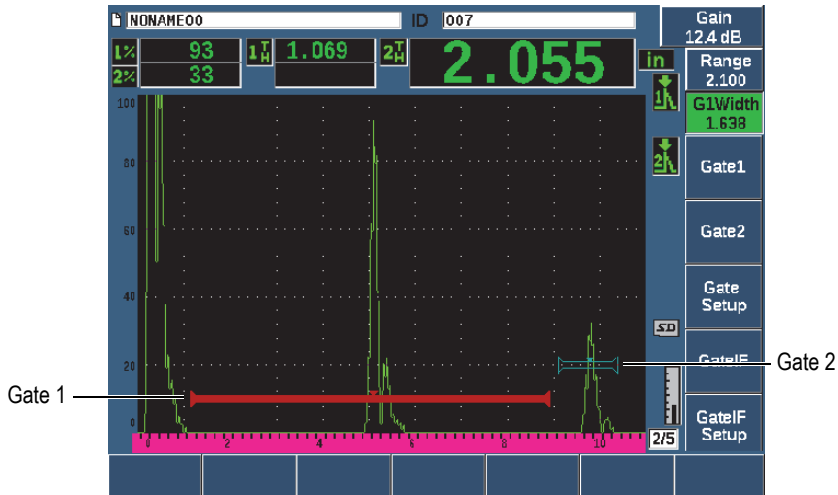
Figure 4-8 Example of an A-scan waveform with gates
