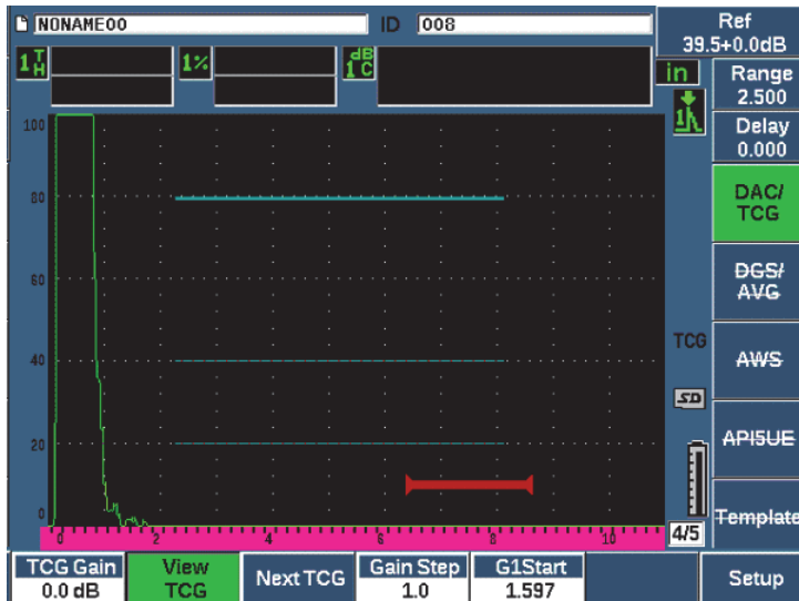
Figure 11-7 Completed DAC curves in TCG view mode
