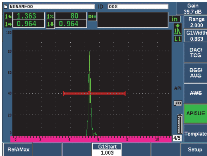
Figure 11-25 Storing the A_{\max} point
